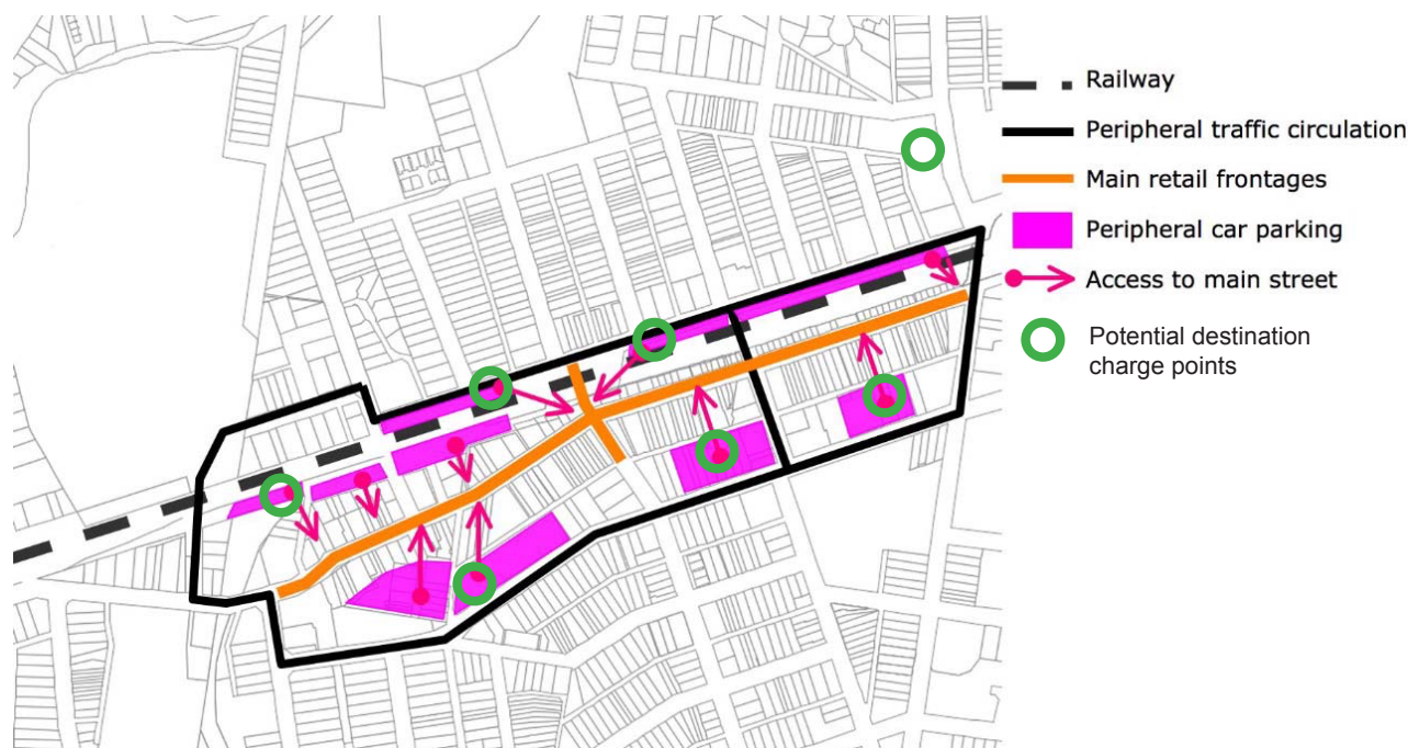
Figure 4 Locations suitable for destination charge points within the Lithgow Main Street precinct
