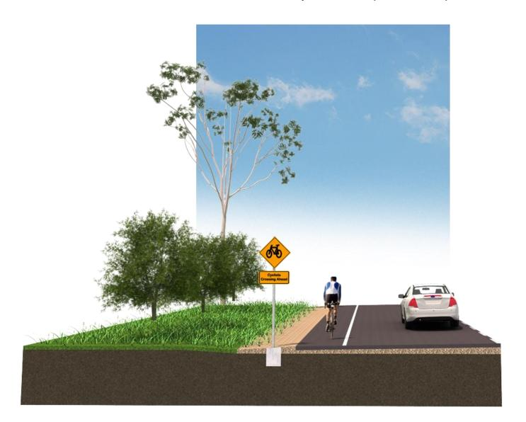
Concept Drawing - Typical on-road 3 m wide shared path design, including 500mm buffer
