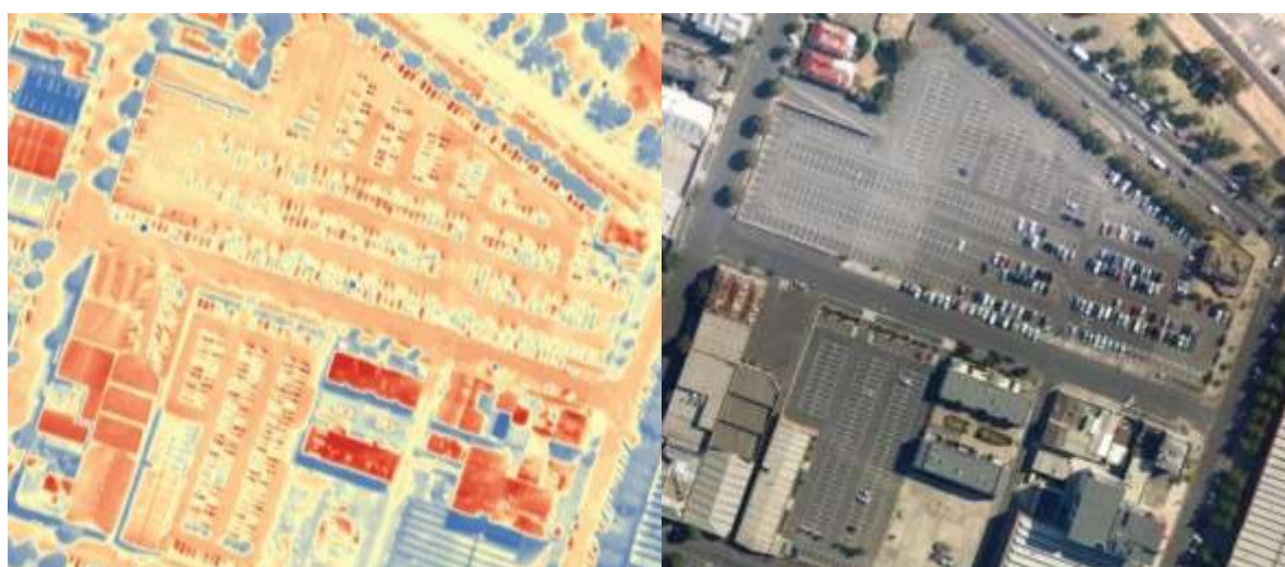
Figure 7: Thermal imagery measurement of surface temperatures at a precinct level (AECOM Australia Pty Ltd, 2013)
