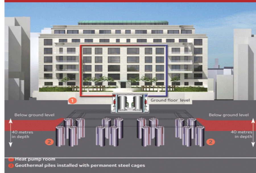
FIGURE 59: EMBASSY COURT – HEATING AND COOLING FROM GEOTHERMAL HEAT PUMP SYSTEM SOURCE: BUILDING.CO.UK
